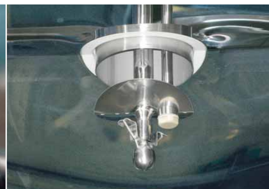
Internal cleaning via high-performance rotating spray head with rotation control
